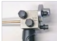
STEP 1: Insert tubing, set depth, and tighten.
