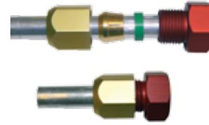
1. Lightly lubricate tube end. Slide nut and correct tubing size brass ferrule (fit will be snug) on tube, threads and taper on ferrule facing end of tube. Allow 1.5" of tube to stick out past ferrule.
