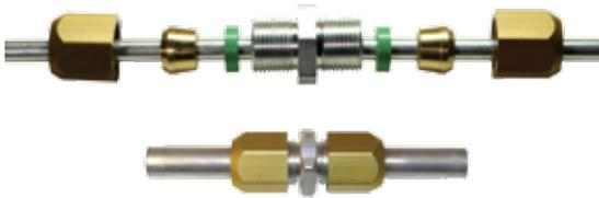
1. Lightly lubricate tubing ends. Slide nut and correct tubing size brass ferrule (fit will be snug) on each tube, threads and taper on ferrule facing ends of tube. Allow 1.5" of tube to stick out past ferrule.
